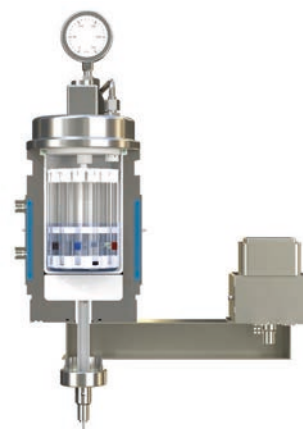
Diagram of Milestone Single Reaction Chamber technology
